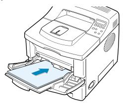
If you want to print on previously printed paper from the Multi-Purpose Tray, the printed side should be facing down with an uncurled edge to the printer. If you experience problems with paper feed, turn the paper around.
